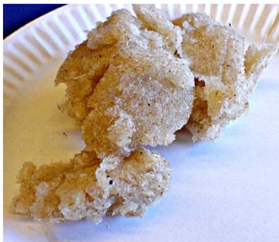
Figure 5: HUSK + 50 mL of water - JUST HOLDING TOGETHER
