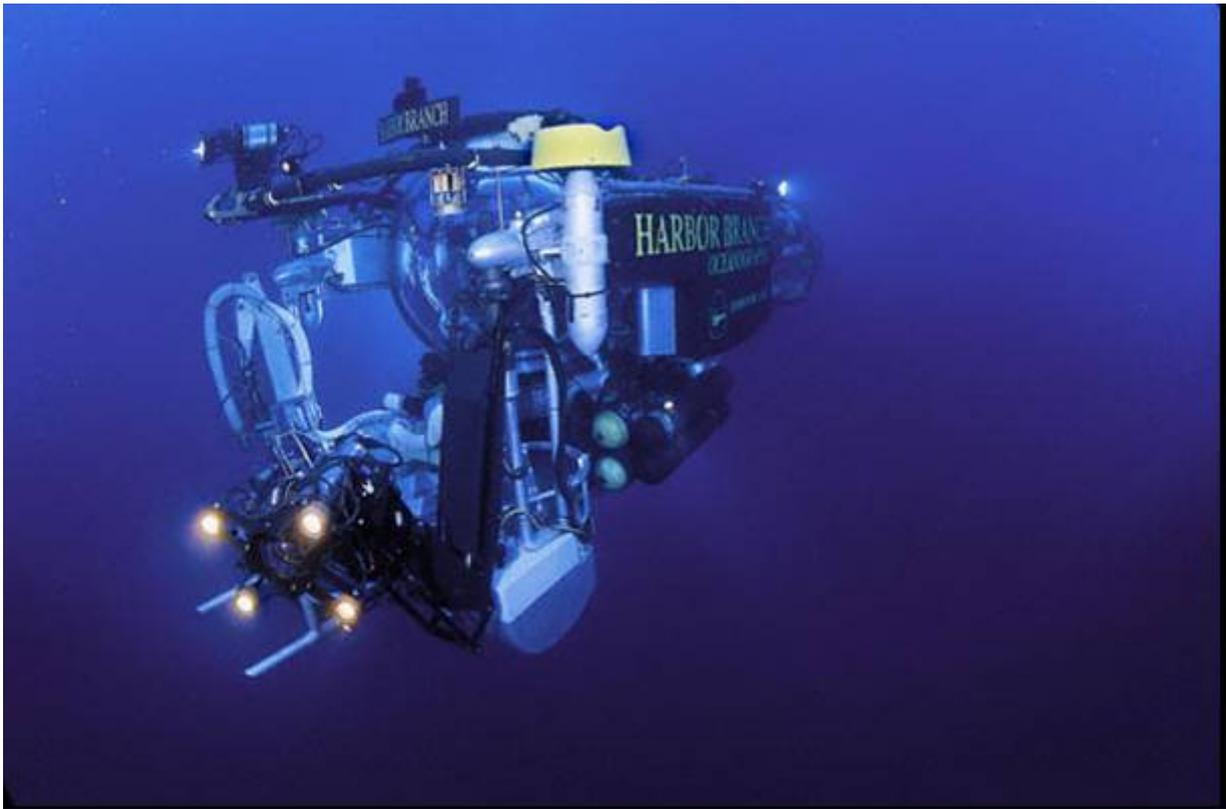
**Figure 5.** A side view of the Johnson-Sealink manned submersible. It has a depth limit of 1000m and the front acrylic sphere (approx 2m in diameter and 12.5cm thick), holds a pilot and observer and provides all-round visibility. A high resolution TV camera with four lights is mounted at lower right and the flexible hose is part of a sampling system that can suck specimens from the water (or the seafloor) and deliver them to storage containers for return to the surface (photo: HBOI)
