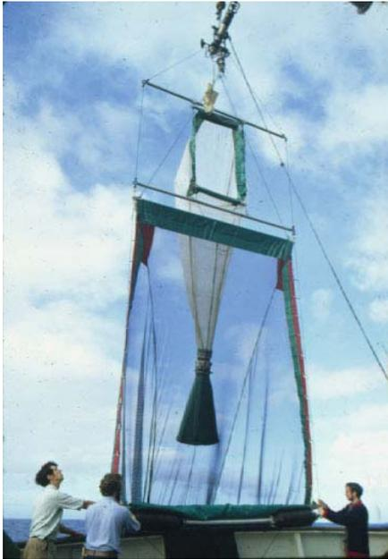
**Figure 2.** An opening/closing Rectangular Midwater Trawl system (RMT1+8). The lower net has an 8m<sup>2</sup> mouth area and mesh of 4.5mm, the upper one a mouth area of 1m<sup>2</sup> and a mesh of 0.33mm. This combination allows a wider size range to be sampled than would be possible with a single net. The nets open and close simultaneously on receipt of an appropriate acoustic signal from the ship. (Photo: Southampton Oceanography Centre)
